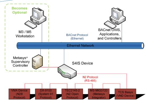
The S4IS BACnet-N2 integration offers flexibility and cost savings when integrating legacy Metasys® N2 networks to Open BACnet Systems. The BACnet-N2 Integration avoids, or defers, costly replacement or re-engineering of existing devices on legacy Metasys® N2 buses.
