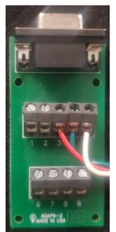
The N2+ conductor uses terminal 3.
